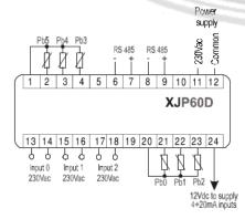
Pb3.Pb4 e Pb5 are configurable as digital inputs free voltage.
