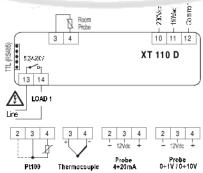
Power supply 24Vac/dc: connect to the terminals 10-12
